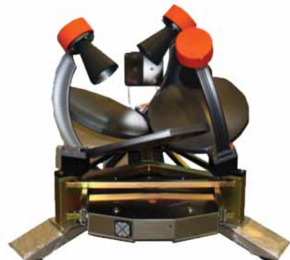
Picture: AQ510 Speaker and Electronic assembly
